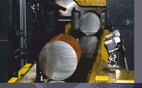
In January 2019 an ultra-modern dividing Linsinger line was installed in the company Vítkovice Cylinders, member of the Cylinders Holding group. New device substantially increases billet breaking capacity and improves the efficiency of the seamless pressure cylinders extrusion node. The saw allows to divide steel billets with a diameter of 150 to 240 mm.
